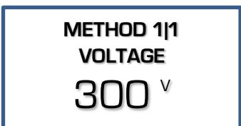
When performing a Voltage gradient, enter the desired end Voltage. The start Voltage is the end point of the previous step. This is 0 V when programming the first step as gradient step.
