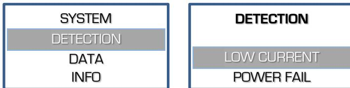
2. Decide whether or not the output Voltage should shut down at a too low output current and press ✓.
