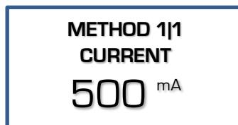
This limit is automatically set to its maximum and cannot be changed in case of a Voltage gradient step.
