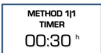
The value format is **hh:mm** when entering a value in hours (**h**). The kiloVolthours (**kWh**) are entered as a value with two decimal places.
