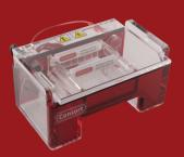
RapidCast™ gel casting technology is ideal for most small gel units with trays that are approximately equal in width and length. The dimensions of all cast-in-place gel trays are adjusted so that when the tray is placed cross- ways in the gel tank, the gasketed ends of the gel tray fit precisely against the walls of the buffer chamber. This forms a leak-proof seal for quick gel pouring.
