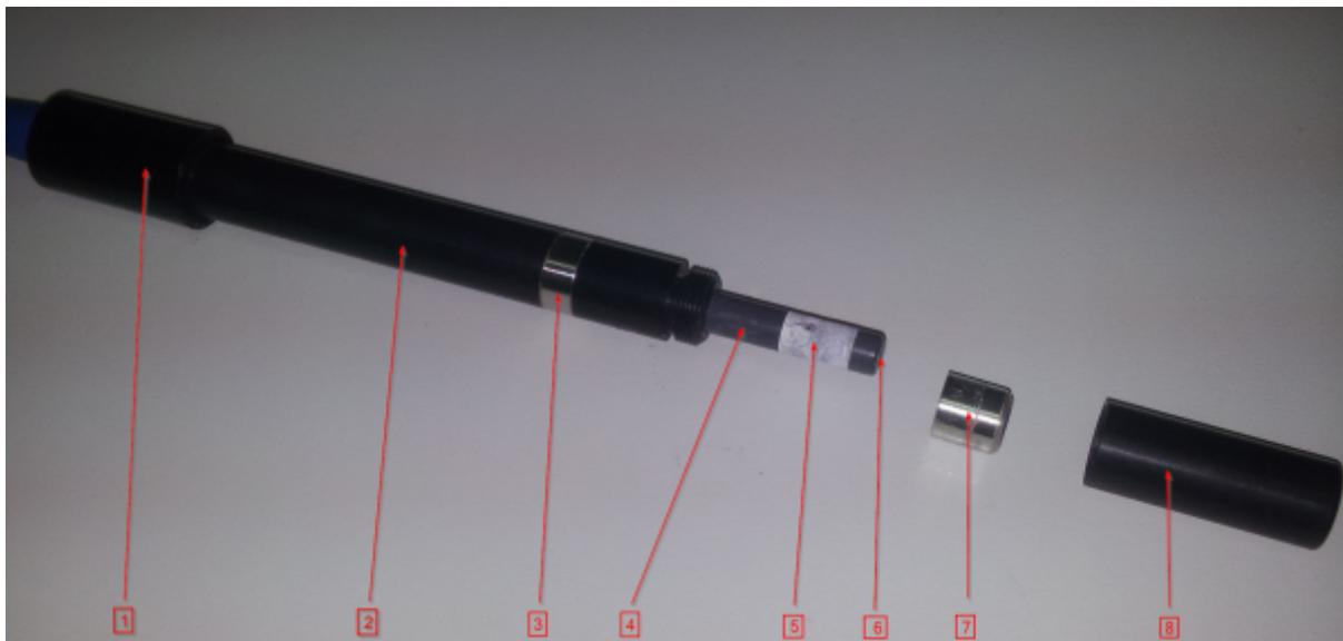
1. Electrode cap (material Nylon) with cable/body connection
