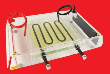
This IEF system has been designed to perform all flat bed IEF techniques, including wick-based electrophoresis with horizontal and hand-cast IEF gels, and focusing with IPG strips.
